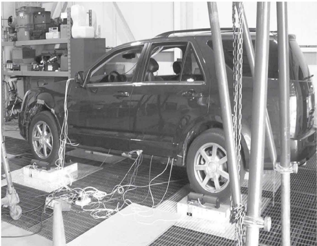
Figure 6-42 A Cadillac SRX 2005 model on a four-post shaker test facility (author's research on active suspension system).
